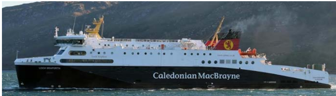
MV Loch Seaforth IMO 9665437. Construction started 16/9/2013 by Flensburger, Germany, Yrd No 764 for Caledonian MacBrayne. launched 21/3/2014, 116X18.4 mts, 7,800 grt, 700 passenger, 143 cars, She is seen on her regular service inbound to Ullapool from Stornoway. Photo: iain Forsyth (c)
