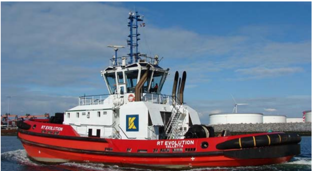
The KOTUG-SMIT operated hybrid tug RT EVOLUTION operating in the port of Rotterdam Photo: Peter Andriessen www.tughunter.nl (c)
