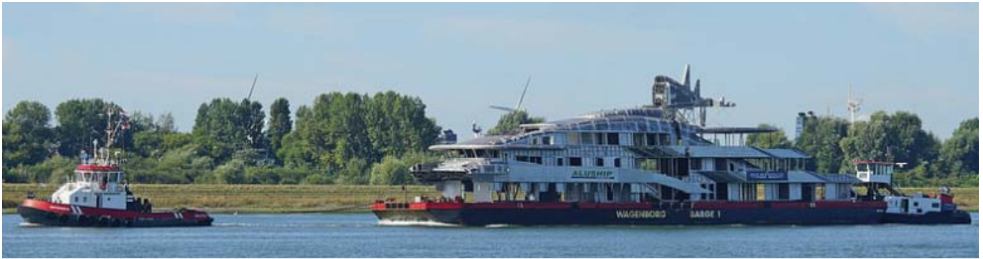
WATERGEUS towing the WAGENBORG BARGE 1 loaded with a superstructure for Aluship assisted by the NJORD inbound for Oceanco in Alblasserdam Photo: Kees Torn © CLICK at the Photo !
