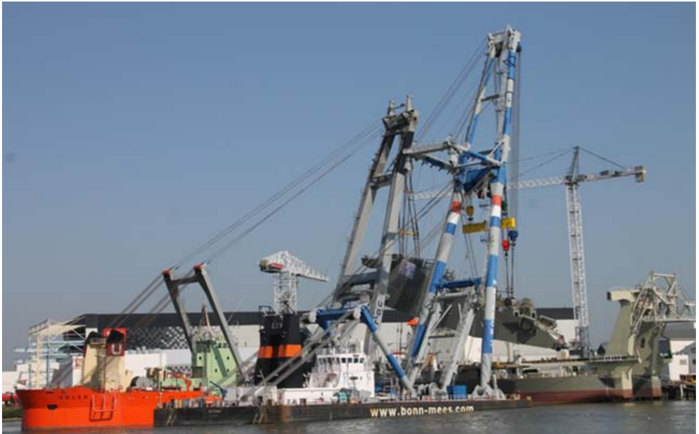
The Sheerlegs MATADOR-3 and UGLEN seen lifting the new cutterladder with a weight of 1717 tons onboard the new Boskalis CSD HELIOS at the Royal IHC shipyard in Kinderdijk Photo: Arie Boer ©
